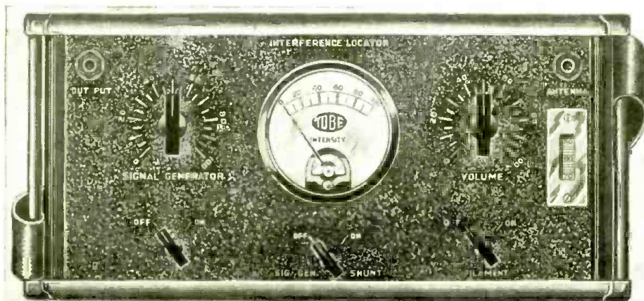
Fig. B Photograph of the panel of the interference locator showing the location of the controls
